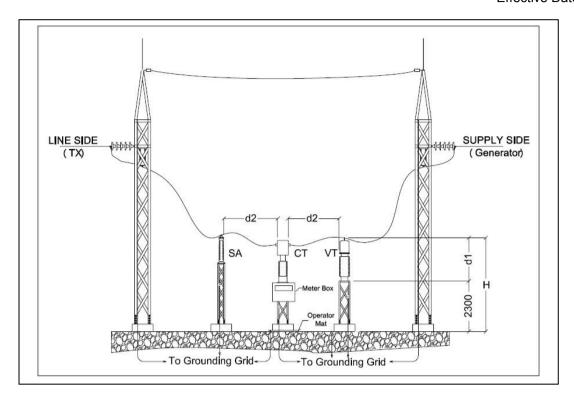
Figure 2(a) - Location/Arrangement of Instrument Transformers (Generator)
