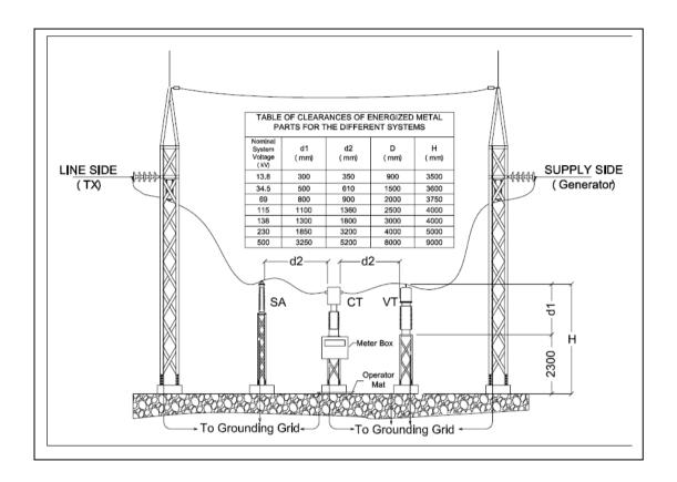
C – TOWER PLAN (DISTANCE BETWEEN INSTRUMENT TRANSFORMERS)
