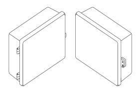
Figure 1 – CT/VT Secondary Terminal Box
