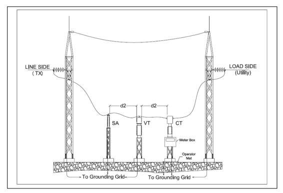
Figure 2(b) - Location/Arrangement of Instrument Transformers (Distribution Utility)
