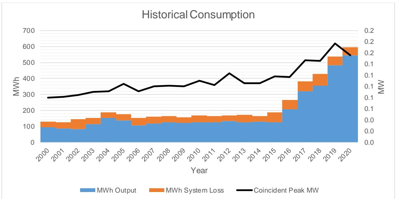
MWh Output increased from year 2001 to year 2020 at a rate of 6.73%, while MWh System Loss decreased at a rate of -1.10% within the same period.
