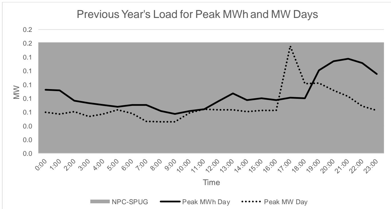
Peak MW occurred on 17:00 due to the residential based energy usage in the island. Peak daily MWh occurred on 21:00 due to residential based energy usage in the area. As shown in the Load Curves, the available supply is higher than the Peak Demand
