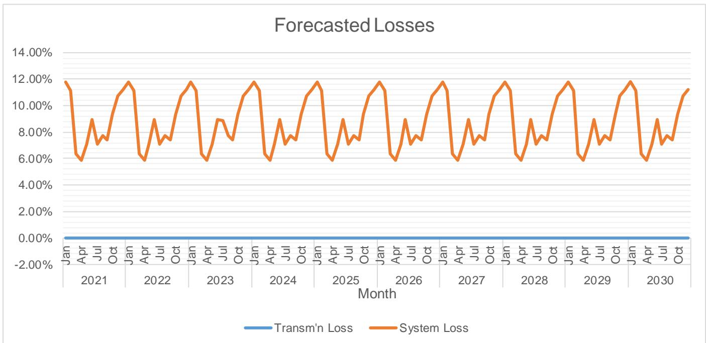
Transmission Loss is expected at 0% while System Loss is expected to range from 5.87 % to 11.81 %.
