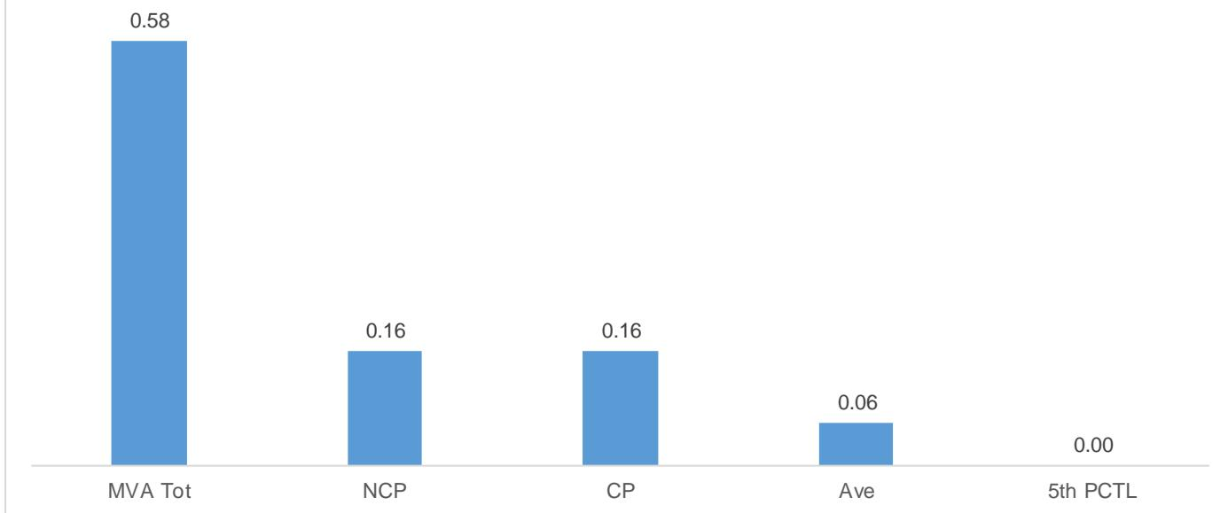
The Non-coincident Peak Demand is 0.16 MW, which is around 27.58% of the total plant capacity of 0.58 MVA at a power factor of 0.275. The load factor or the ratio between the Average Load of 0.06 MW and the Non-coincident Peak Demand is 37.5% of. A safe estimate of the true minimum load is the fifth percentile load of 0 MW which is 0% of the Non-coincident Peak Demand.
