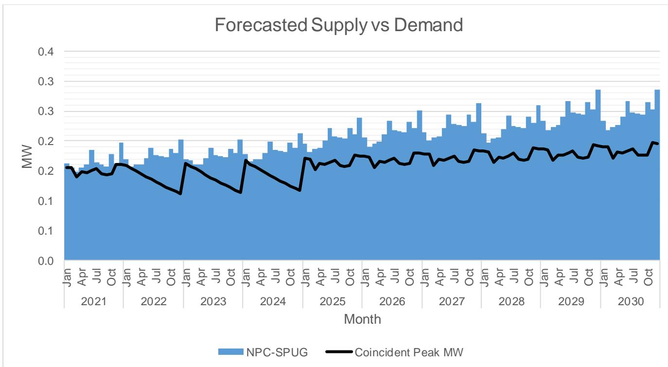
There is only single available supply, of 0.58 MW plant capacity from NPC-SPUG (Hikdop Island).
