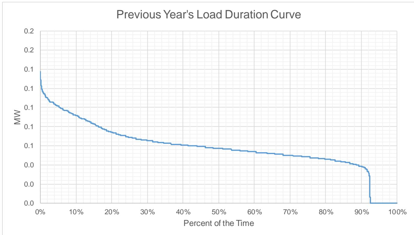
Based on the Load Duration Curve, the minimum load is 0 MW and the maximum load is 0.156 MW for the last historical year.
