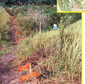
Sound waves reflected from the sub-surface are picked up by an array of geophones (receivers) which are laid out on the ground along a seismic line and connected to recording instruments through a seismic cable.
