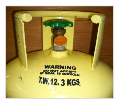
Check if the security seal is intact and firmly affixed to the Pressure Relief Valve (PRV).
