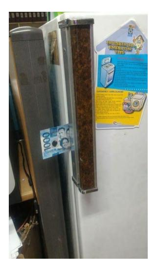
Do the **"BILL TEST"** to test if the Magnetic Lining of the Ref's door is still working properly.
