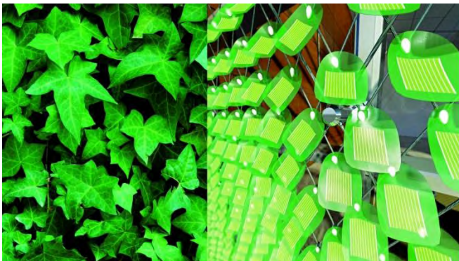
Solar Cell Layout based on Vine-leaf arrangement
